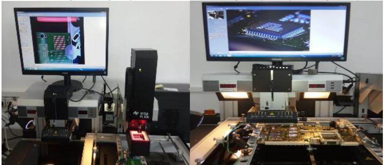
-1 station for soldering-detaching components with infrared heating, with precise positioning of components
