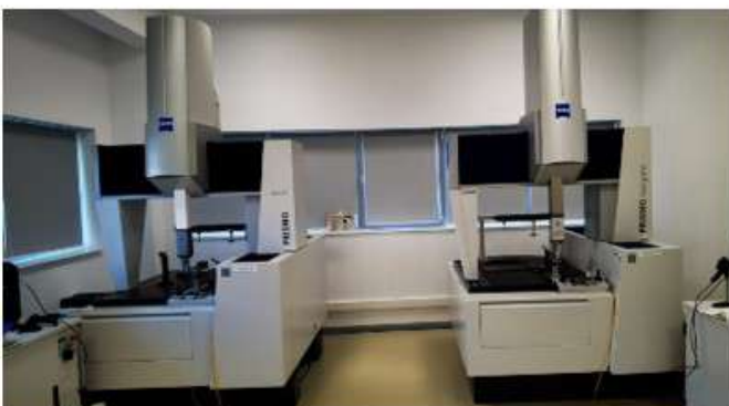
Fig. 1 CMM Zeiss (COMPAs has 20 machines available for complex measurements)
