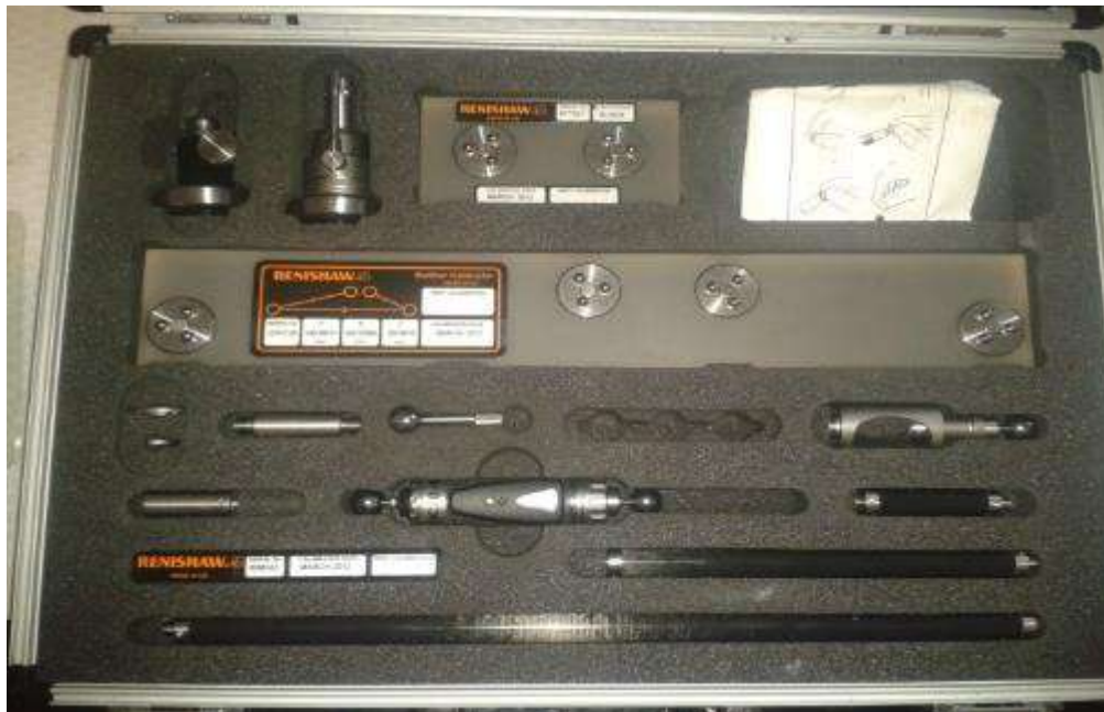
c. Qualitative analysis of the machine tool axis geometry, carried out with the Renishaw QC20 BallBar toolkit.
