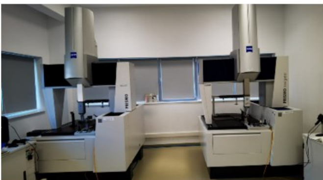
Fig. 1 CMM Zeiss (COMP A has 20 machines available for complex measurements)
