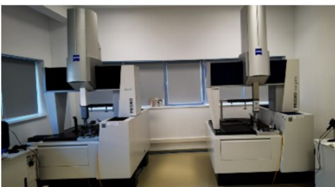
Fig. 1 CMM Zeiss (COMP has 20 machines available for complex measurements)
