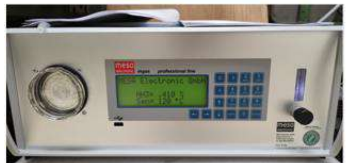
Fig. 8 Ammonia gas analyzer
