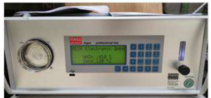
Fig. 8 Ammonia gas analyzer
